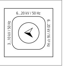
Fig. 2: Voltage selector switch (only Art. No. 767 416)
