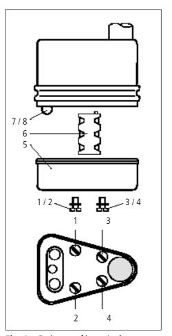
**Fig. 4:** Exchange of batteries/lamp
