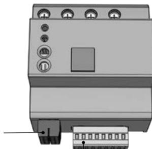
A slotted screwdriver (≤ 2.5 mm) is required to unlock the push-in connectors
