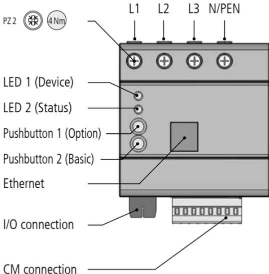
**Attention!** Current sensors must be connected to the device **before** mounting on the current conductor!
