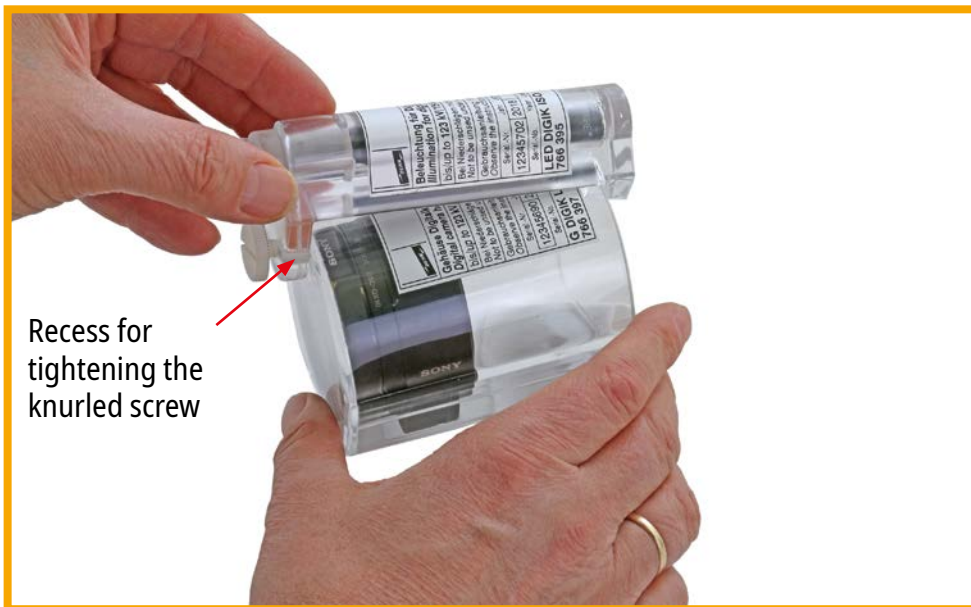
Fig. 5 Attach LED housing to camera housing
